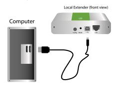
4 Attach the USB device(s) to the REX.
