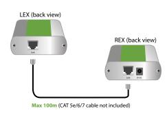
Connect the REX to the AC adapter and plug it into a power source.
