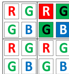
Figure 8-48 Horizontal and vertical color Binning by 2x2
