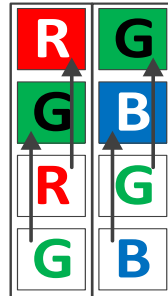
Figure 8-47 Vertical color Binning by 2
