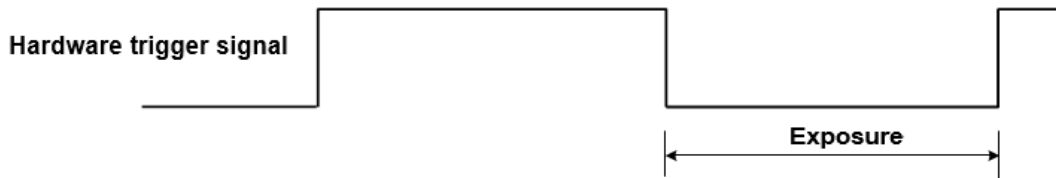
Figure 8-30 The sequence diagram in falling edge trigger of TriggerWidth exposure mode
