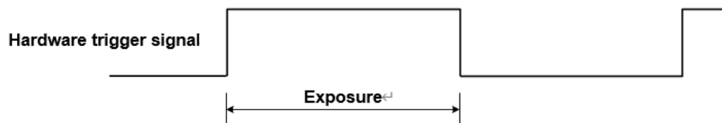
Figure 8-29 The sequence diagram in rising edge trigger of TriggerWidth exposure mode
