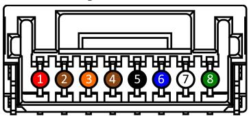
GPIO connector as seen from rear VQ GigE series view. Pin colors correspond to GPIO-8P20 cable from Vieworks.
