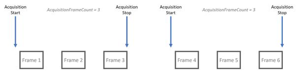
Under MultiFrame acquisition mode, frames are acquired once AcquisitionStart is called. The number of frames acquired is dictated by the parameter AcquisitionFrameCount. During the acquisition process, all Transport Layer parameters are locked and cannot be modified.
