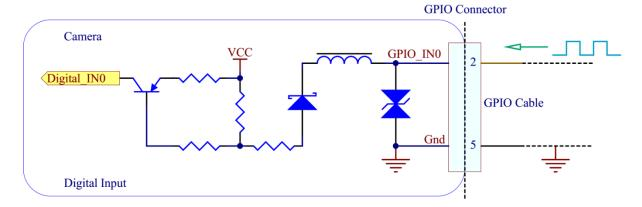
Non-isolated Input Measurements:
