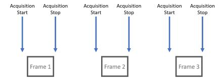
Under SingleFrame acquisition mode, one frame is acquired after AcquisitionStart is called. AcquisitionStop is an optional call as the acquisition process automatically stops after the single frame is acquired. During the acquisition process, all Transport Layer parameters are locked and cannot be modified.
