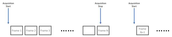
Under Continuous acquisition mode, frames are acquired once AcquisitionStart is called. Frames are acquired until AcquisitionStop is called. During the acquisition process, all Transport Layer parameters are locked and cannot be modified.
