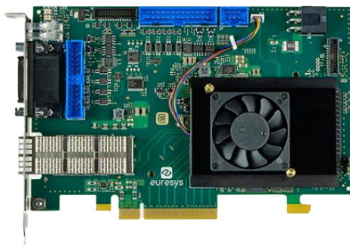
Figure 4-1 Good Frame Grabber to Use Together: Coaxlink QSFP+ from Euresys
