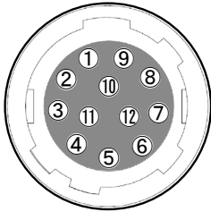
Figure 7-4 Pin Assignments for Power Input and Control I/O Receptacle
