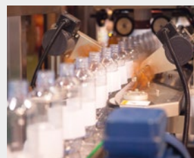
Label inspection on containers with different dimensions in the cosmetic, healthcare and beverage industries.
