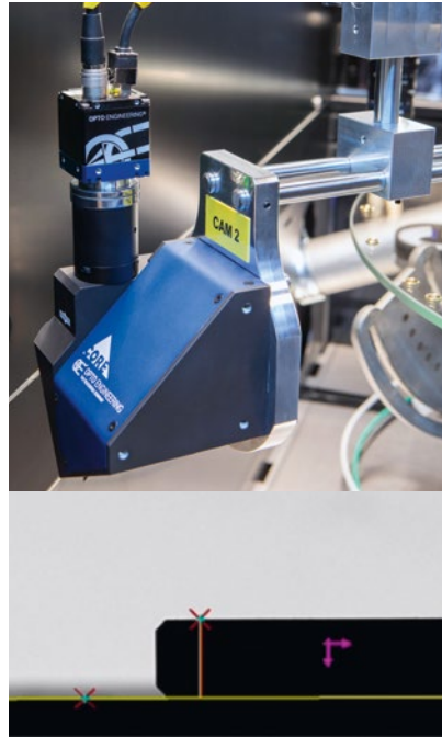
A 12MP camera measures the height combined with a CORE telecentric lens and a telecentric illuminator.
