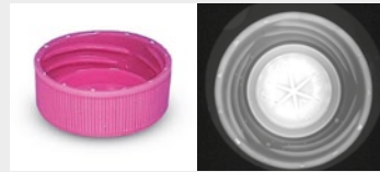
Inspection of plastic bottle caps for thread and shape defects.
