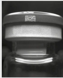
A 5MP camera combined with a 2/3" fixed focal optics with liquid lens performs OCR and data matrix reading.
