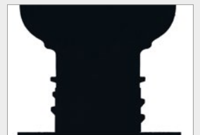
Dimension control of plastic bottles and preforms up to 200 mm in diameters with TC2MHR CORE lenses.
