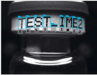
A 5MP camera combined with a 2/3" fixed focal optics with liquid lens performs OCR and data matrix reading.
