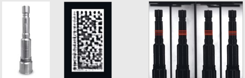
A 5MP camera reads the data matrix and measures the nozzle diameter with a TCCAGE lens.
