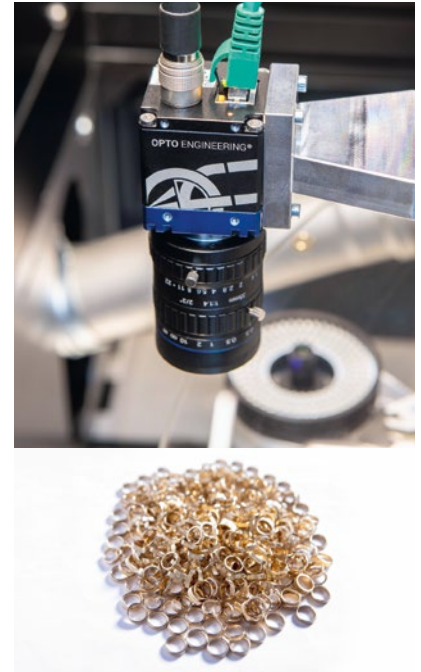
A 5MP camera with a 35 mm fixed focal lens inspects surface defects or processing residuals.
