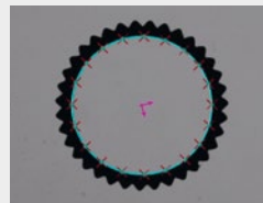
Measurement of automotive cogwheels with a TC3MHR telecentric lens.
