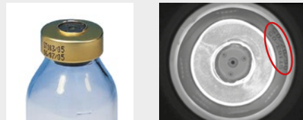
The expiration date can be easily read without the need to know the bottle orientation.
