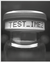
A 5MP camera combined with a 2/3" fixed focal optics with liquid lens performs OCR and data matrix reading.
