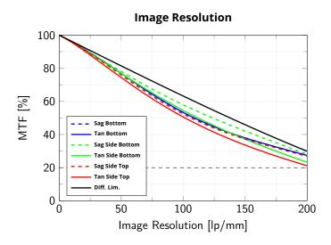
Modulation Transfer Function (MTF) vs. Image Resolution, wavelength range 486 nm - 656 nm, wf/N, of cylindrical object of diameter 30 mm and height of 20 mm
