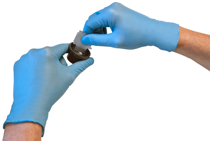
Figure 8: Second step: release the mount ring.
