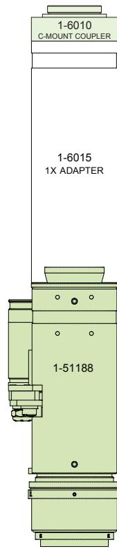
12X Zoom configuration with right angle adapter and motorization
