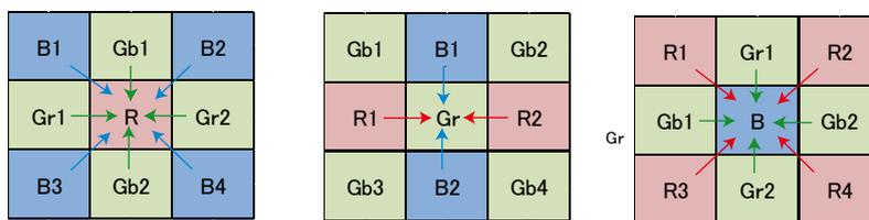
Fig.40 Color interpolation concept drawing
