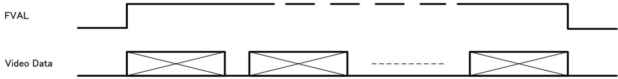
Fig.17 Horizontal timing (Timing inside the camera)
