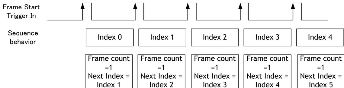
Fig. 29 Behavior of Sequence trigger
