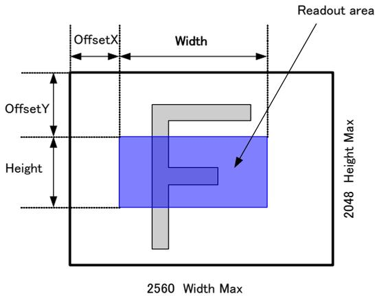
Fig. 21 Setting example (No binning)
