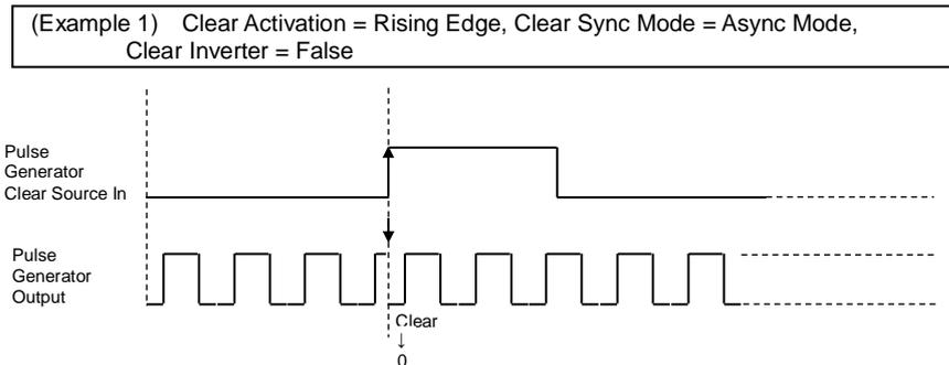
**Fig.12 Counter clear in Async mode**
