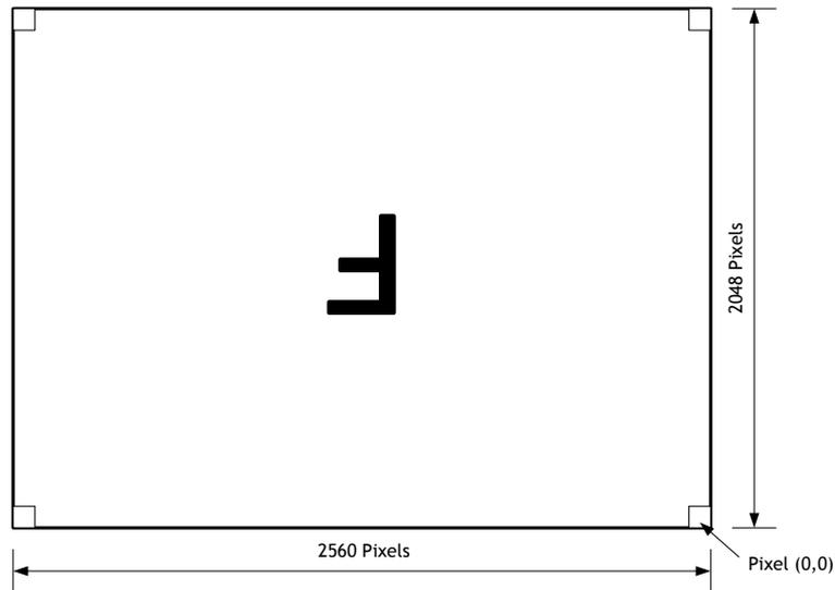
Fig.14 Monochrome sensor layout
