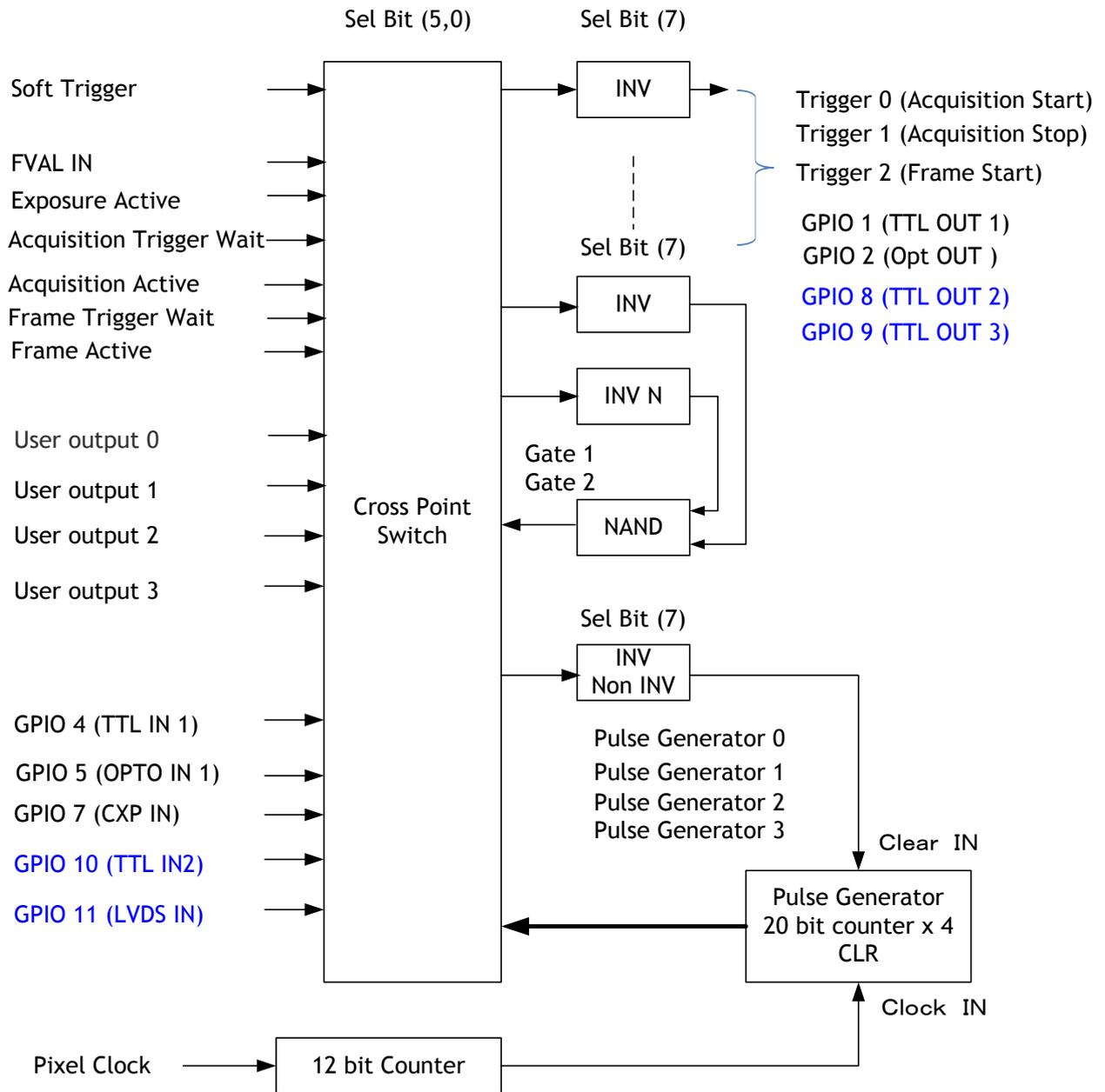
Note1: The pixel clock is 86.4 MHz.
