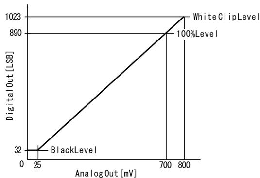
Fig.23 Bit allocation (10-bit)
