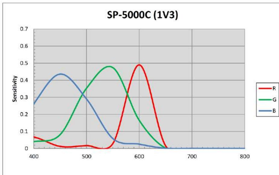
Fig.45 Spectral response (SP-5000C-CXP4) (With IR Cut Filter)
