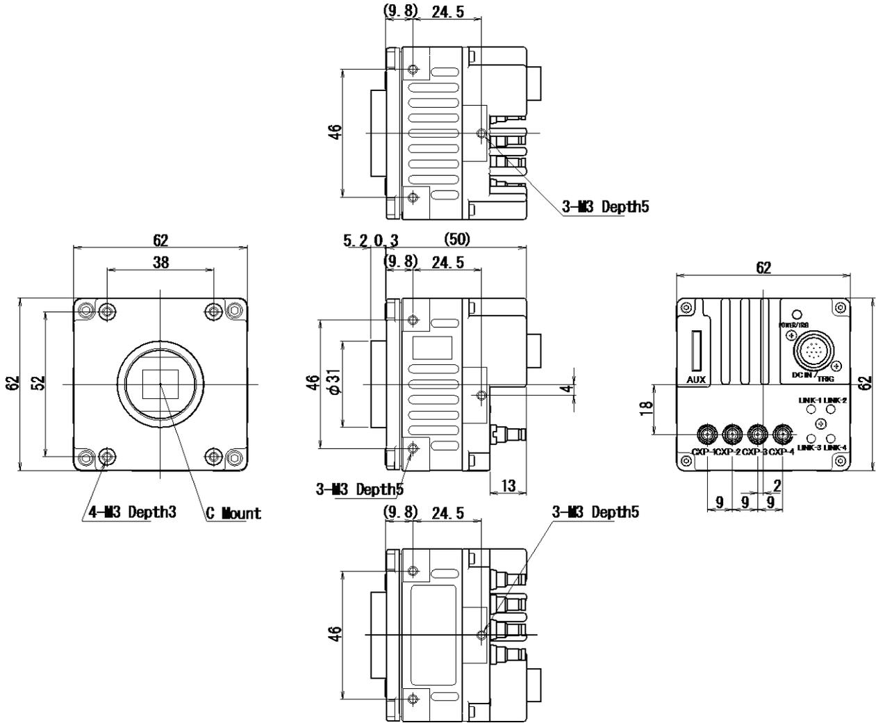
Dimensions tolerance:  $\pm 0.3\text{mm}$
