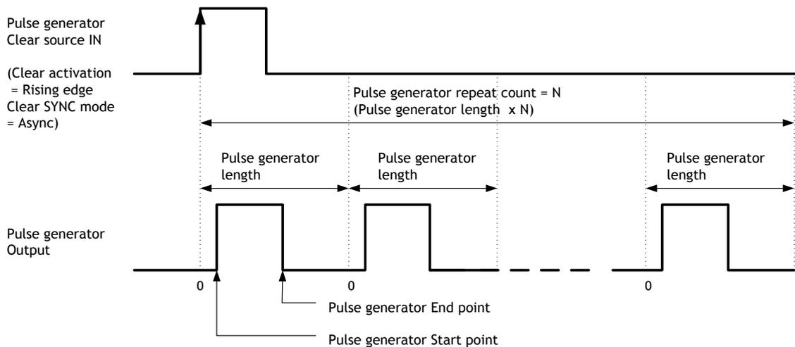
**Fig.11 Pulse Generator pulse construction**
