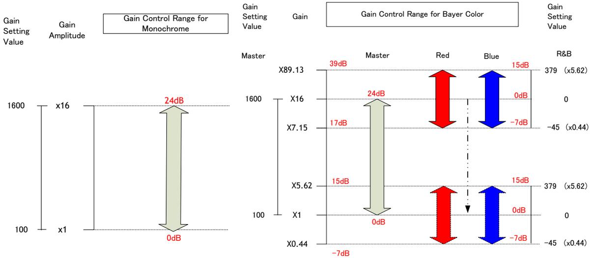
The above drawing shows the relationship between gain setting value (command), gain amplitude, and dB indication. For example, the gain amplitude “x 0.44” equals -7dB.
