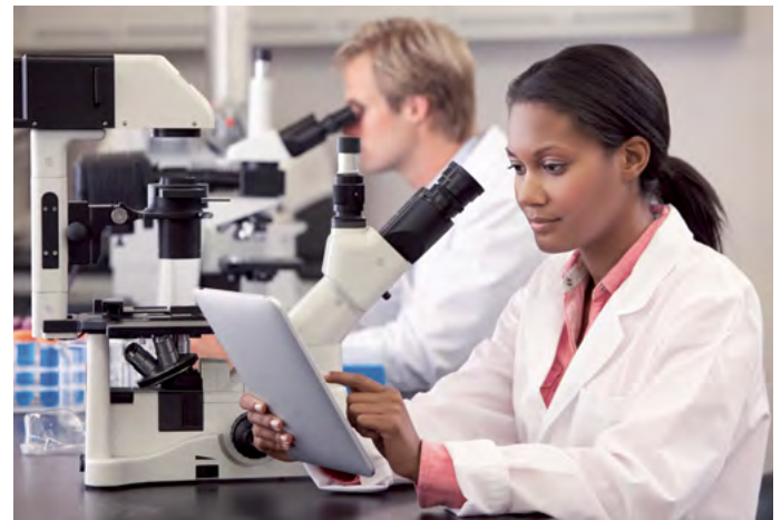
Typical microscopy workstation for routine laboratory applications with a binocular inverted microscope (front) and an upright microscope (in the background).
