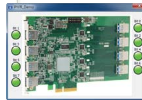
Auxiliary function API for software-programmable per-port power on/off control
